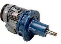
achieved by loosening the (4) mounting bolts that secure the motor to the reducer. If the gear is too loose, simply tap the motor in, toward the center of the reducer. Check the play in the gears and continue the process until the desired tolerance is achieved.
