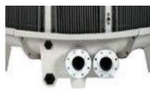
OF THE PIPING ON THE TOWER FLANGES. It is recommended that the piping be supported no more than 18" from the actual tower connections. Failure to do this could cause damage to the tower bulkhead and void the warranty.
