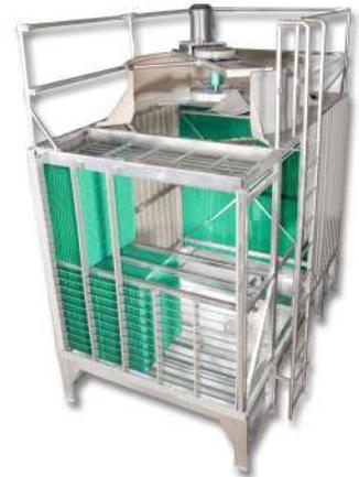
**1.1 FRP COMPONENTS:** The hot water basins, cold water sumps, side panels and fan stacks, are constructed of non-corrosive FRP (Fiberglass Reinforced Polyester). This material is light weight, very durable and impervious to the effects Rust, Water Treatment Chemicals, Hard Water or Biological attack. The exterior panels are treated with UV inhibitors to prevent damage due to long term sun exposure.
